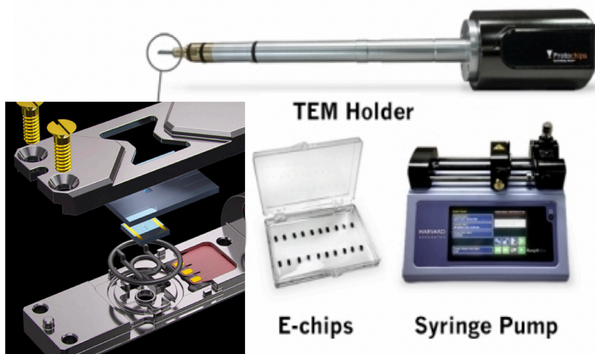
Figure 1: Schematic of a ProtoChips Poseidon Liquid Cell TEM holder. http://www.protochips.com
